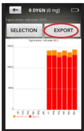
4. In order to save the information on your PC proceed as follows. Connect MyFID<sup>®</sup> to the PC's USB port using the cable from MYFID<sup>®</sup> package. Select on the MyFID<sup>®</sup> which format you would like to transfer the data with CSV is a format that various spreadsheet programs e.g. Microsoft Excel can open. If you select "Export PDF report", you get a standardized
